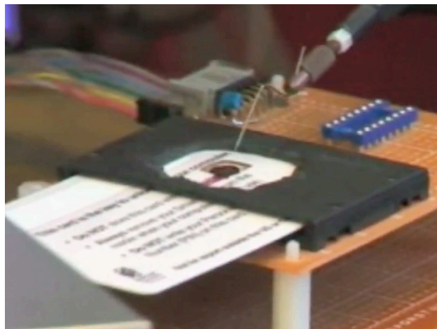
Probing a smartcard die using a micropositioner and angled sewing needle (from Wired's Hack a Sat-TV Smart Card video 16 ).
