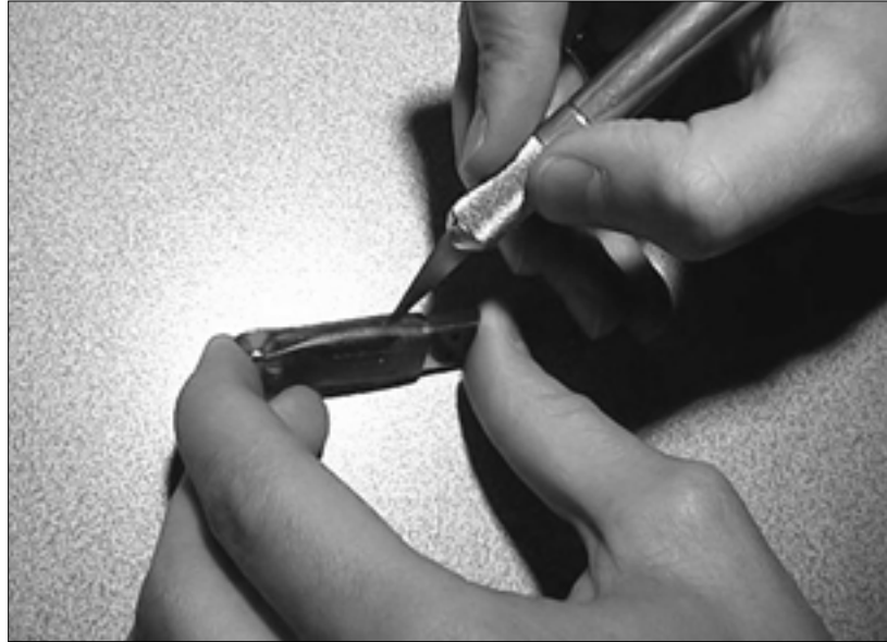
Figure 14.1 Opening the Housing of an Authentication Token Device with a Simple X-Acto Knife
